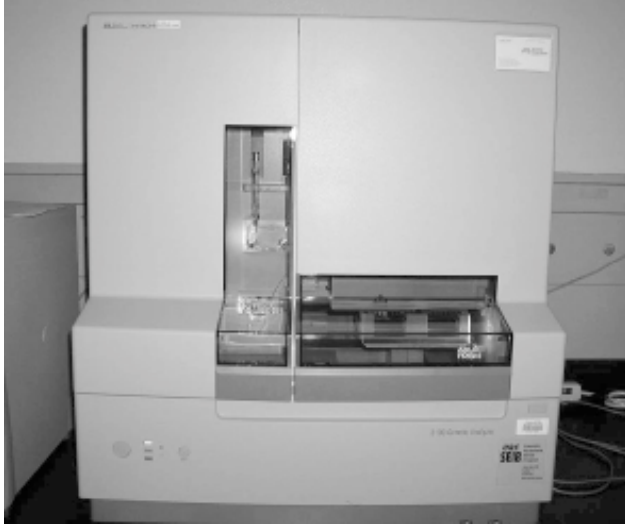
Figure 7. The ABI PRISM 3100 ® Genetic Analyzer used to generate sequence data for high-throughput processing of family references. Validation is in progress for usage on sequencing degraded skeletal remains samples.
