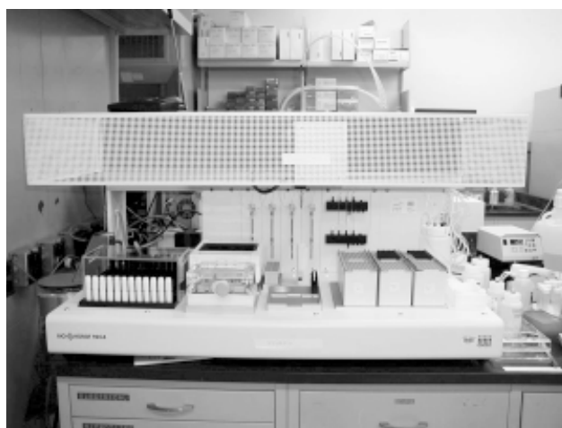
Figure 6. The Qiagen BioRobot ® 9604 (Qiagen: Venlo, The Netherlands) used for the high-throughput processing of family reference samples.
