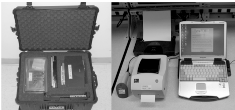
Figure 1. LISA Mobile. On the left is the “Go-Kit” contained within the travel kit. Each piece of the kit has a cushioned slot. Each LISA Mobile kit contains supplies to collect approximately 1000 specimens. On the right is LISA Mobile in operational mode.
